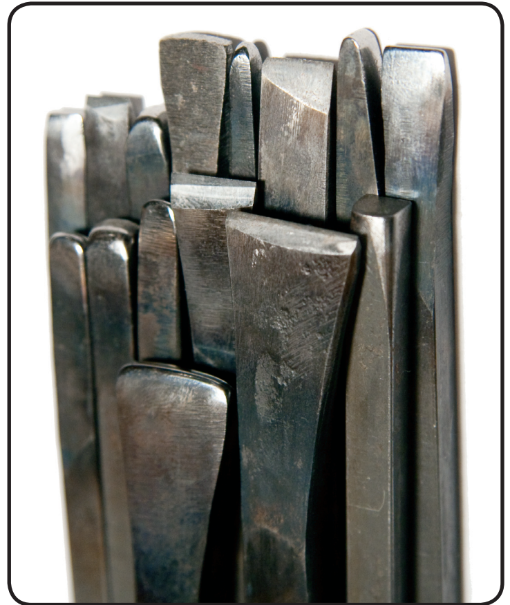
A fistfull of chasing punches of various sorts. Some are chisels, some are liners and others are formers.
