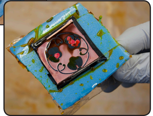
Sample piece after 15 minutes. Notice the sludge, even with EE, and the etchant trapped under the tape.
