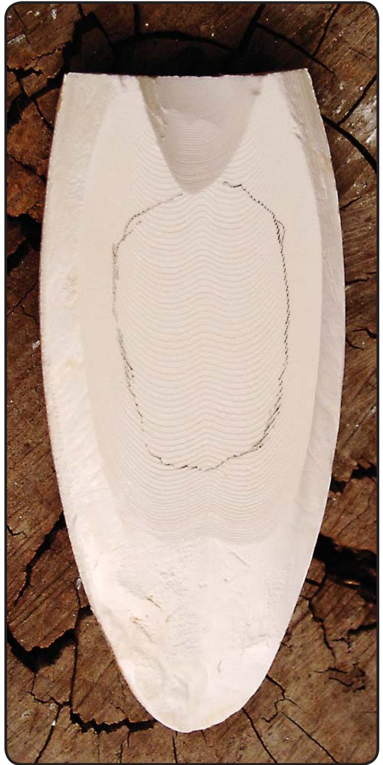
*Cuttlefish bone with flat area and funnel carved in. Note pencil marks indicating 'safe area' to work within. Note that this safe area does not reach all the way to the bottom tip of the bone, as this individual shell became thin at the lower tip. Remember to pay attention to the actual cuttlefish bone in your hands, not just what the handout says you should be able to get away with.*
