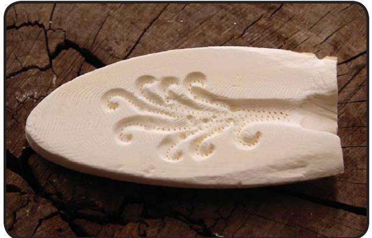
*Another design. Again, notice how the design radiates from a thick area attached to the funnel. Note also the little dots pressed down into the cuttlefish.*
