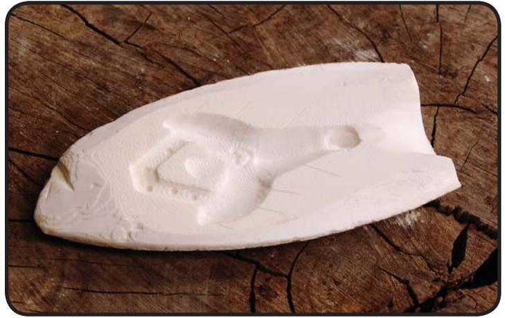
*Cuttlefish bone with design carved, and attached to funnel. Notice how the spine of the design forms a sprue.*
