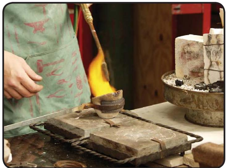
*Melting the metal in a ceramic crucible.*
