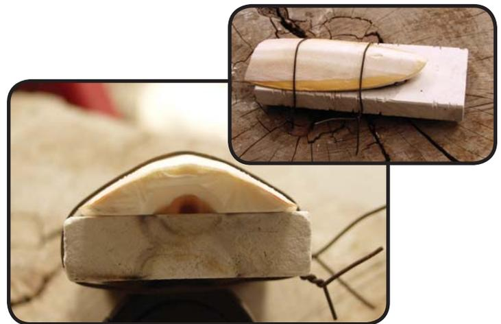
*Cuttlefish wired to soldering board. Not light visible between the bone and board. No light visible through the inside of the mold.*
