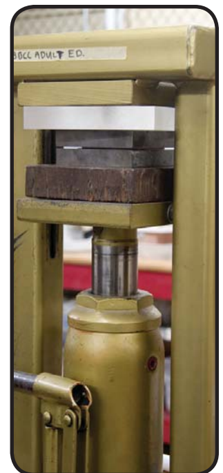
The metal sandwich on a steel surface block, prior to being flattened in the press...
