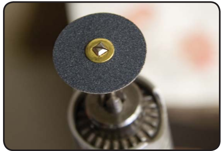
Flex shaft with snap-on sandpaper disk.
