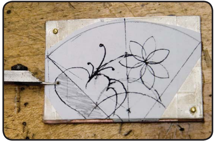
Hole drilled for piercing. Note that it's beyond the area of the fan that I'm planning to use, but that the 'ground' is still completely trapped within the parent sheet.
