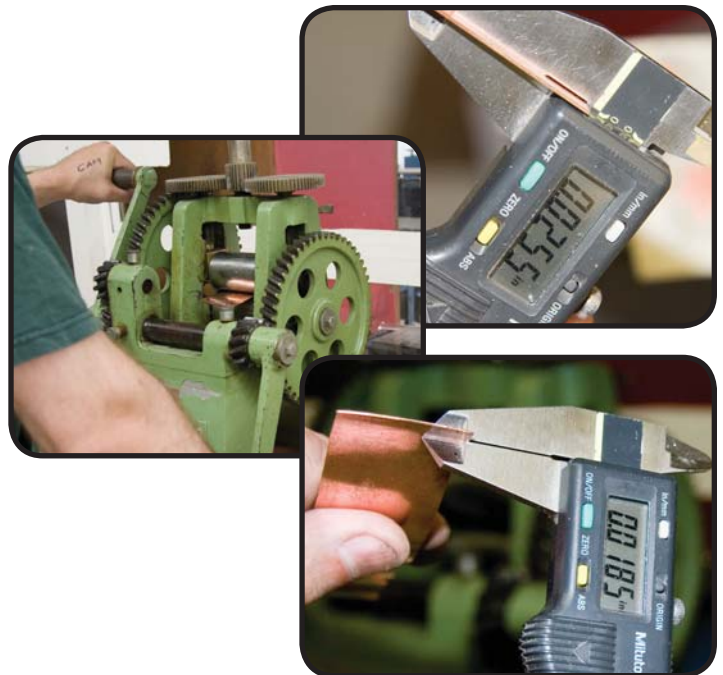
From top: Selecting contrasting metal to make lines. Rolling to thickness. Checking thickness. Tapered bottom edge of metal strip to be inserted into line. The exact angle isn't important. The idea is just to make it thin enough to make it easy to get it into the sawn line.
