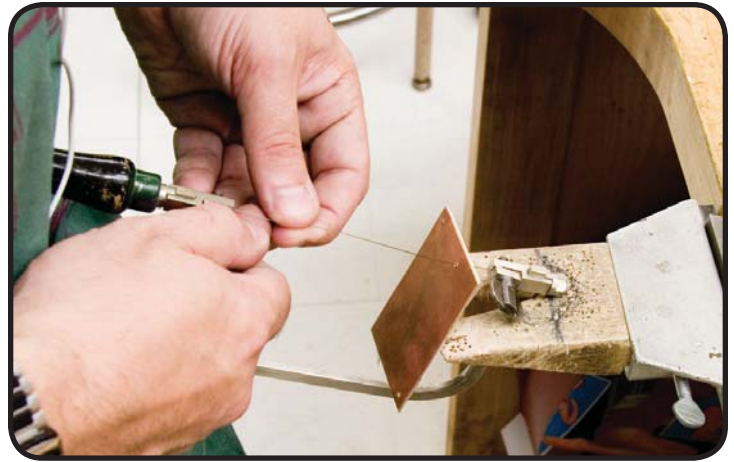
Threading sheet metal onto saw. Note that the metal is all the way up against the forward blade clamp. This will support it, and leave you with two hands to fasten the blade.
