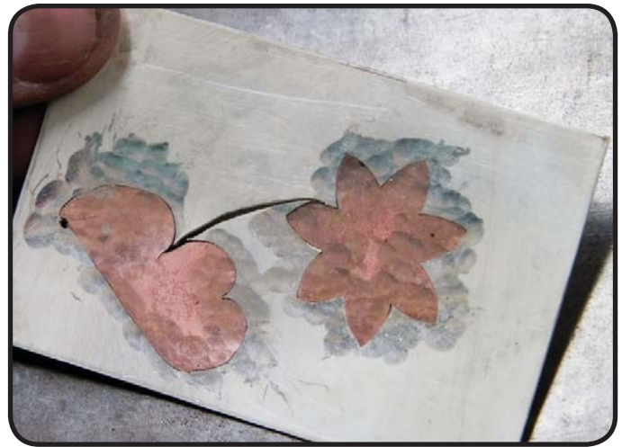
Parent metal with both inserts planished into place. Note that they're tight enough to hold themselves in place.
