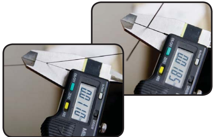
3/0 and #6 saw blades. .011" and .0185" respectively. The different thicknesses of sawblade will give you different line weights of inlay color. Important idea to remember.
