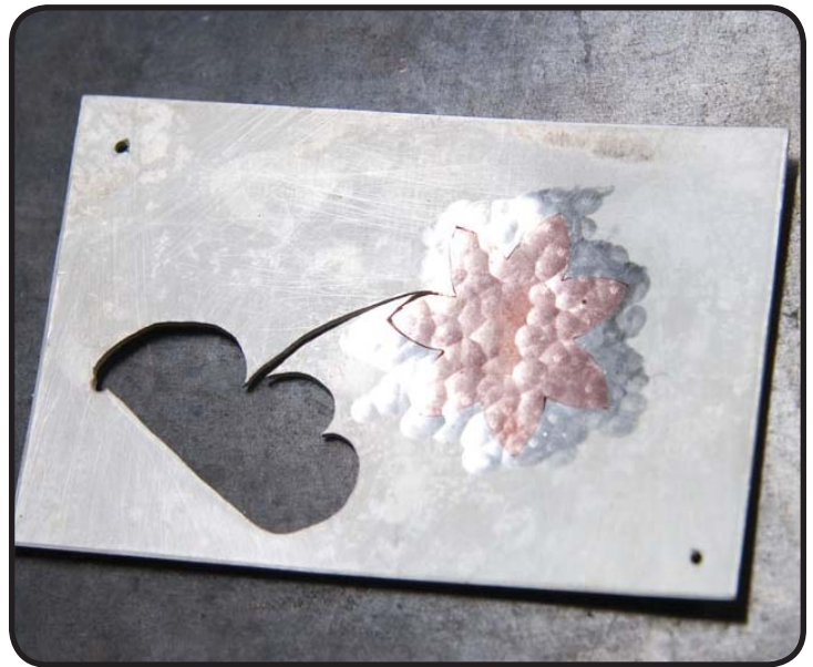
The flower insert planished into place. Notice that I'm only doing them one-at-a-time.
