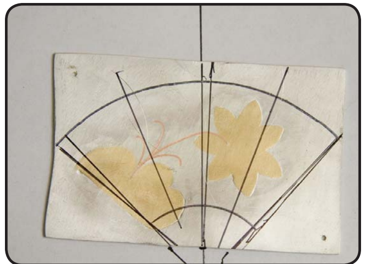
Laying out the pattern for the fan onto the completed sheet of married metal. Note the pattern revisions to maximize material usage.
