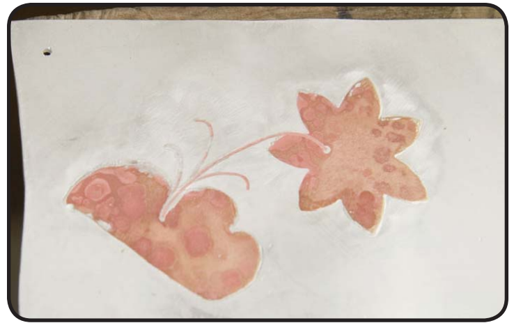
Front side of cleaned up parent metal. Note that lines have been ground flush, as have inserts.
