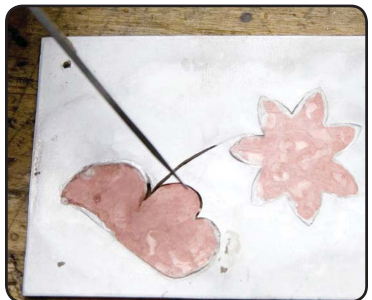
Inspecting the joints after the first soldering pass. The indicated area was replanished before resoldering.
