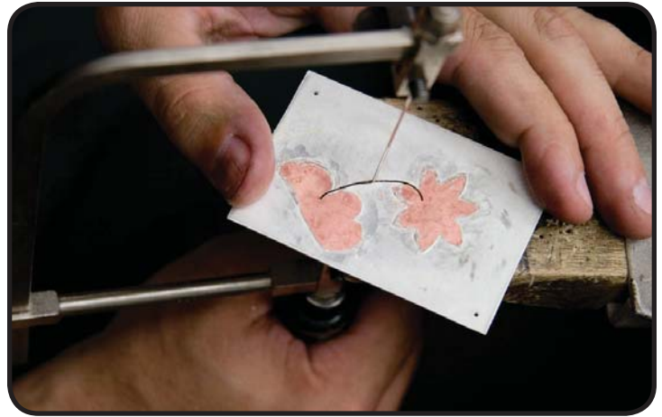
Resawing stem line with #6 sawblade. Note that the line now extends into the inserts. This helps visually unify the design.
