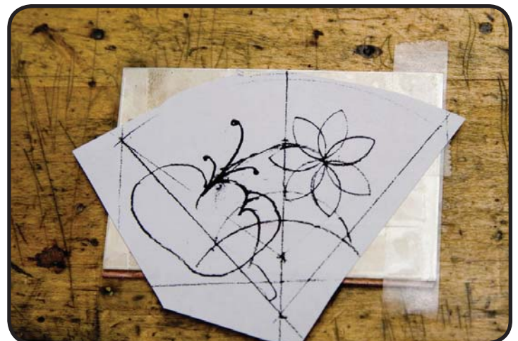
Design, xeroxed and taped onto metal surface with double-sided tape.
