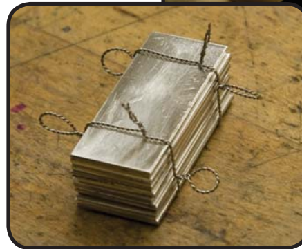
The billet with both wire loops in place. Note the twists of wire on either side, as well as the twist on the top. Try to get them all as tight as possible without breaking the wire.
