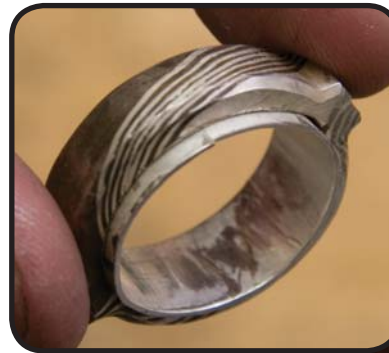
The sleeve inserted into the mokume ring.
