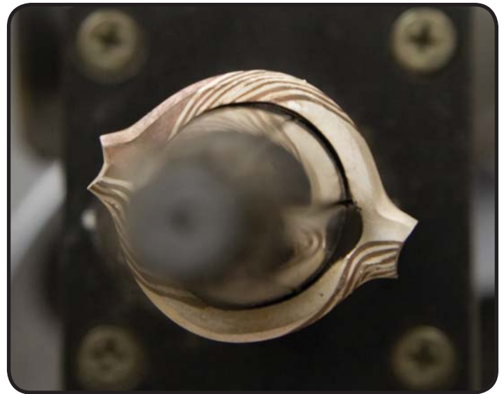
The ring on a mandrel. Note that the drill holes have not completely driven down yet.
