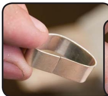
The "under & over" technique for evening out the stresses, allowing the edges to meet evenly.
