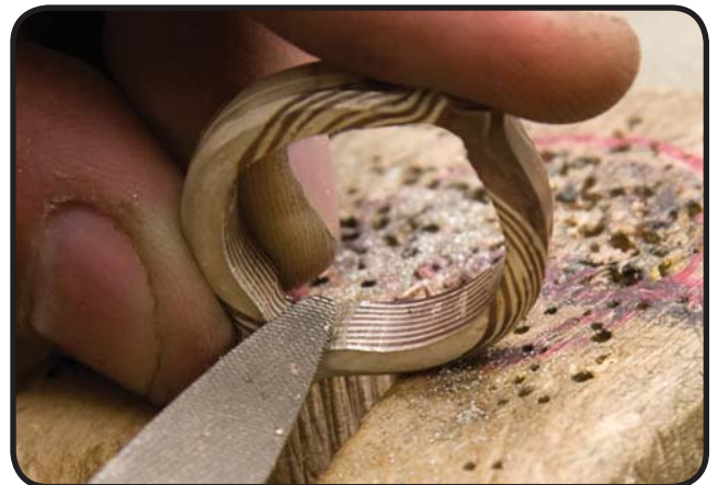
Filing away at the ‘ski-jump’ edges of the drilled holes.
