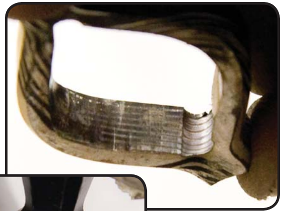
The “ski-jump” steps left behind by the drilled holes
