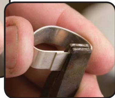
The "under & over" technique for evening out the stresses, allowing the edges to meet evenly.
