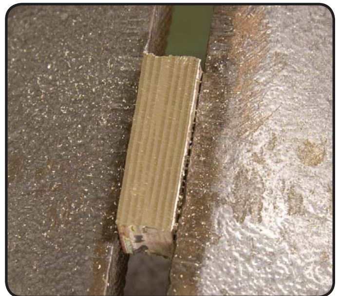
The billet held sideways in a vise. One edge has been filed clean. Note the stripes.
