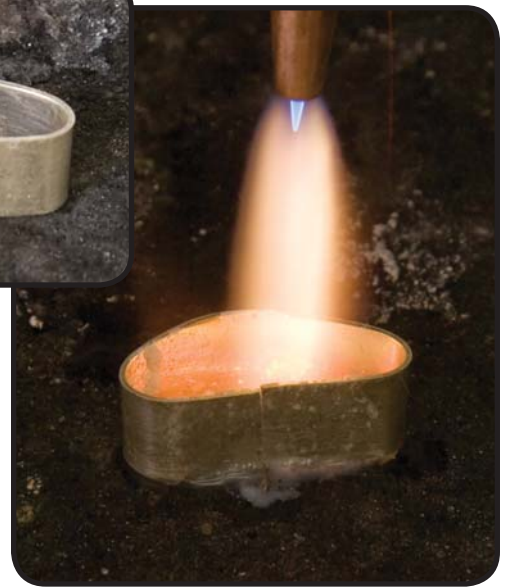
Soldering the sleeve. Note that the torch is firing straight down into the ring.
