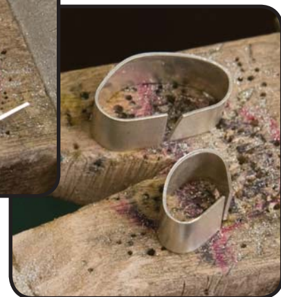
Closed into "D" shapes.
