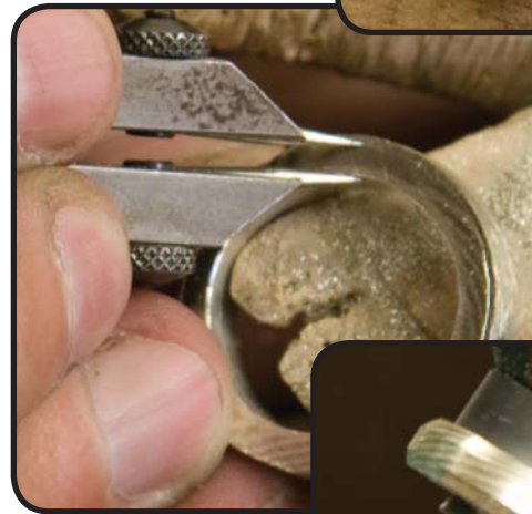
Marking the outside diameter of the ring.
