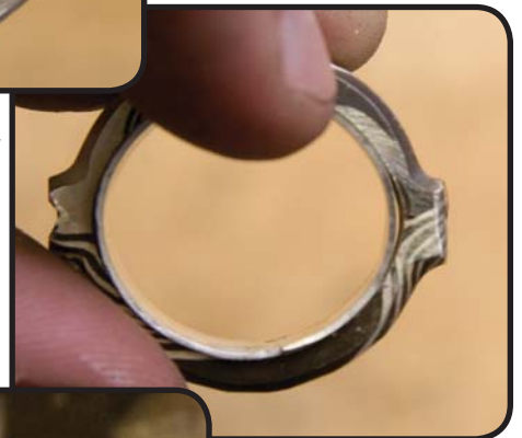
The sleeve inserted into the mokume ring.
