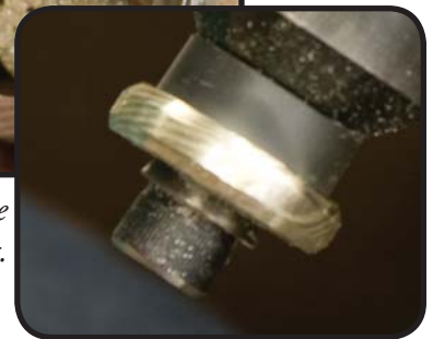
The ring filed with 45° edge bevels.
