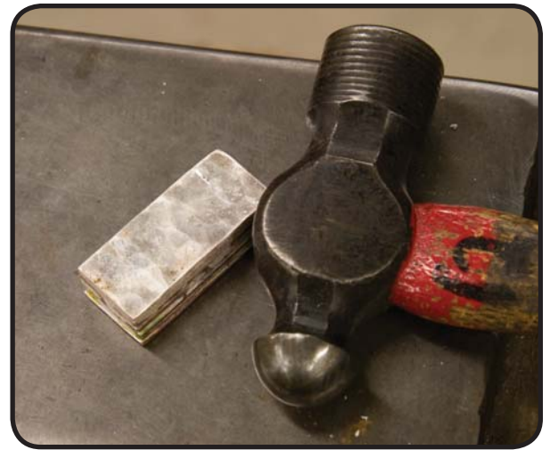
Using the hammer to consolidate the billet. The goal is simply to hammer the whole upper surface.
