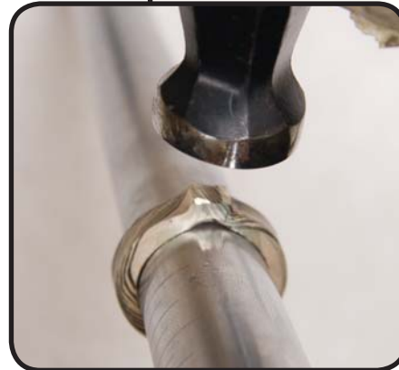
Hammering the stumps down against the mandrel.
