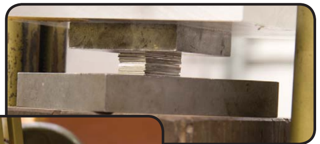
The billet crushed in the press between 2 steel blocks.
