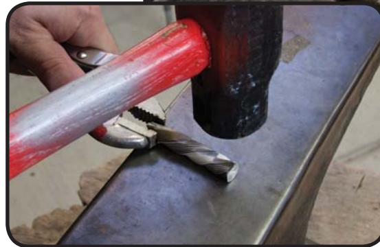
Forging the bar. Note that the visegrips are beyond the edge of the anvil.
