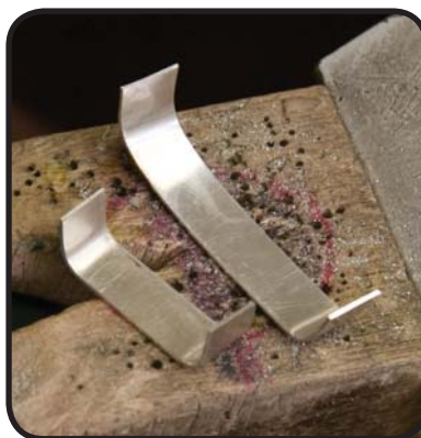
The two strips bent up into staple shapes
