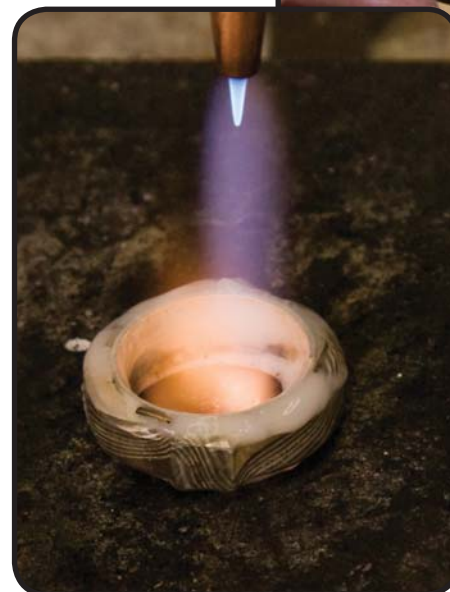
Soldering the sleeve into the mokume ring. Note the torch firing straight down into the ring again. This traps the heat within the ring, heating it more quickly.
