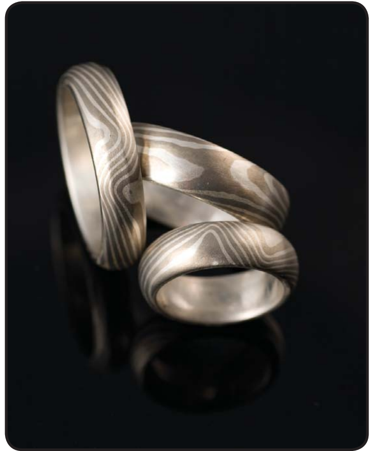
Three finished Mokume-Gane rings. The materials are sterling silver & nickel silver
