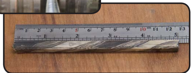
The billet after the second rolling & straightening.
