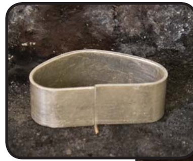
The sleeve before fluxing. Note the position of the solder. The weight of the ring holds it in place until it melts.
