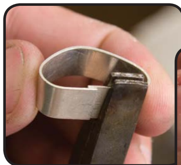
The "under & over" technique for evening out the stresses, allowing the edges to meet evenly.
